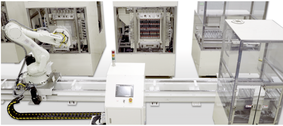
Plating Line Integrated with Automation System
