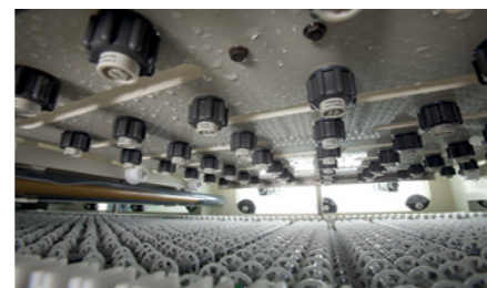
Top: Developing equipment Center: Direct spray, no shadow effect Bottom: Develop spray manifold
