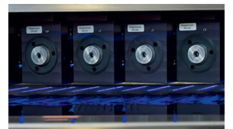
Top: LDI equipment PLI400 SpeedLight Center: Polygon mirror with 48 facets Bottom: Polygon module during exposure
