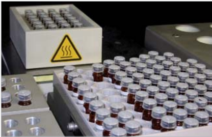
Readily prepared sample vials in auto-sampler racks
