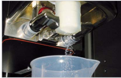
Microdos powder dispensing module for weigh-in of solid samples
