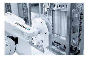
Furthermore, the electroplating equipment adopts a modular design, which can be flexibly configured according to the customer's production capacity and plant area. The components can be quickly operated and disassembled, easy to maintain and can help customers to carry out efficient production.
