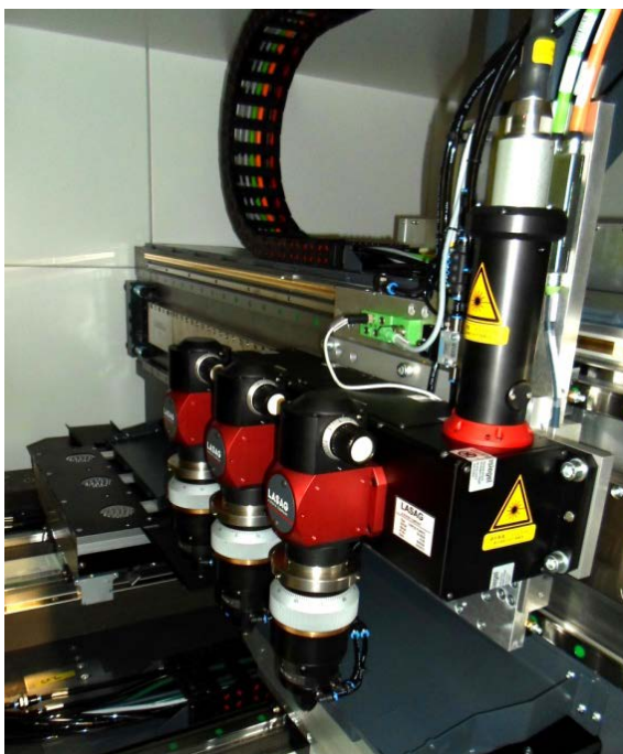
Caption: Multiple cutting heads in a laser system provide maximum throughput and an optimization of operating time.
