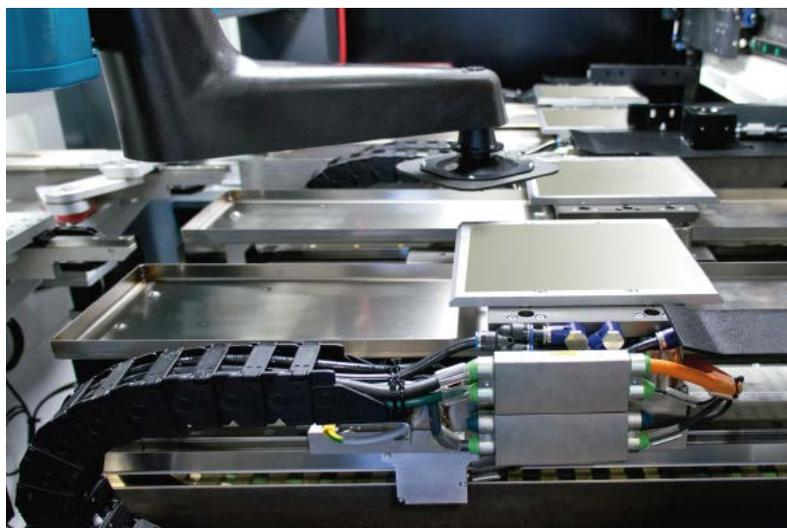
The square ceramic film with an edge length of 130 mm is dropped by a Bernoulli gripper on the table
