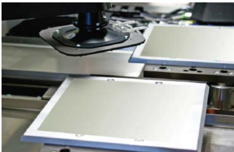
In order to double the throughput, two ceramic films can be processed simultaneously. Therefore, the laser beam is split and directed to two independently controlled scanners
