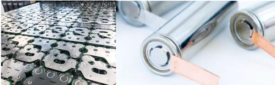
**Image 2:** Cost-efficient mass production only via automation: welded copper conductors with nickel coating on lithium-ion battery packs.
