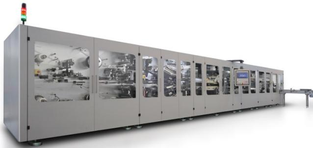
Flexible configuration: The laminating and stacking equipment of the BLA series for laminated and stacked lithium-ion battery cells
