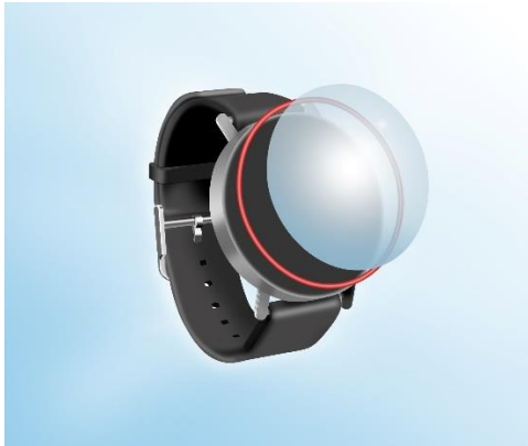
Image 1: Touch Displays on smartwatch housings are sealed water-tight. With this solution from Manz, the red adhesive element is fed fully automatically, activated by laser and then the cover glass is pressed onto it.
