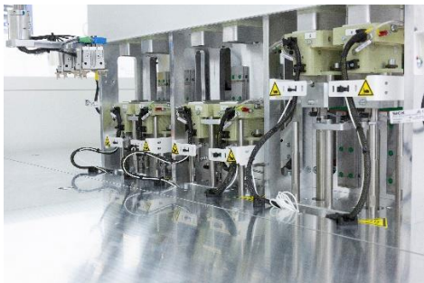
Image 2: Loading interface for the display sealing system from Manz with three alternating and buffered-for-loading pre-tempered press units.
